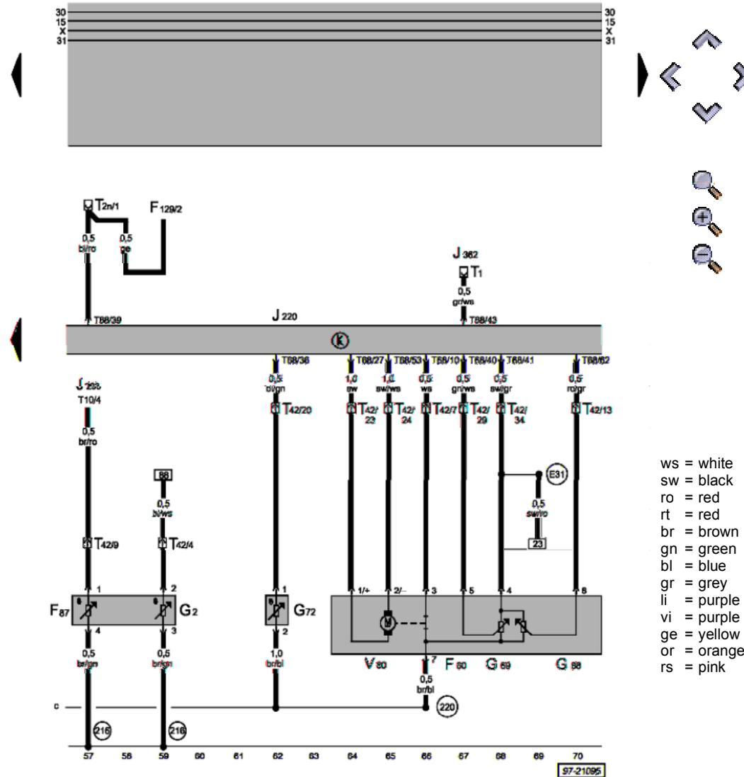
**Motronic control unit, coolant temperature gauge sender, coolant temperature sender, throttle valve control part**
