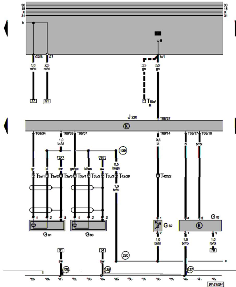
**Motronic control unit, knock sensors, throttle valve potentiometer, intake air temperature sender, air mass meter**
